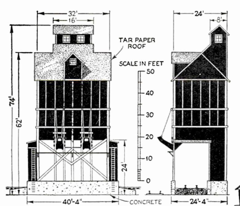
Full-size dimensions in feet are given for convenience in working to any desired scale
